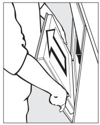
Grip the sides of the door and lift until the hinges disengage. Remove the door.
